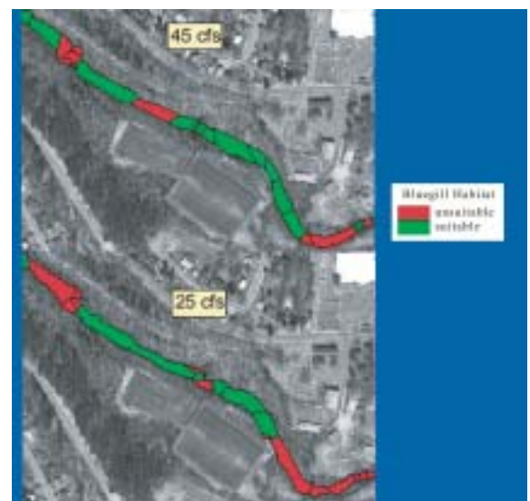
Figure 5: Piotr Parasiewicz shows that fish habitat varies with flow in Hudson River tributaries.
