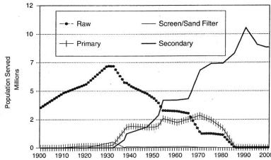
Figure 23.2. Trends of wastewater flow to the middle and lower Hudson River (combined) from ca. 1900–2000, including untreated flows, primary and secondary treatment flows, and total flows.
